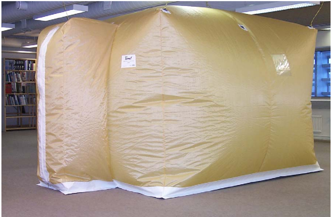
The LSS-80 Protection System deployed. The Protective Tent is pressurized with clean air at 25 Pa positive pressure. Note the viewing window on the tent side wall.
